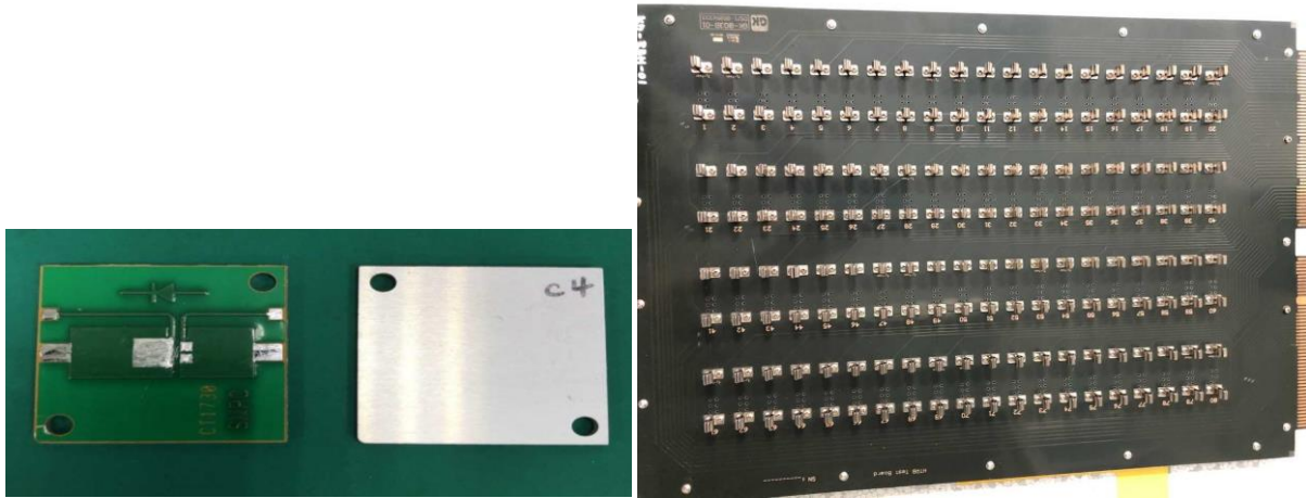
Figure 3: Typical pictures of HTRB test boards
