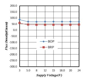
Figure 1. Supply Voltage vs. Flux Density
