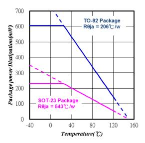
Figure 8. Power Dissipation vs. Temperature
