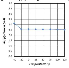
Figure 3. Supply Current vs. Temperature
