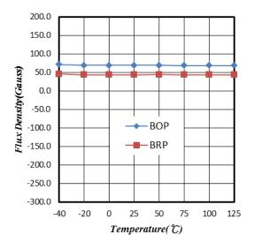
Figure 2. Temperature vs. Flux Density
