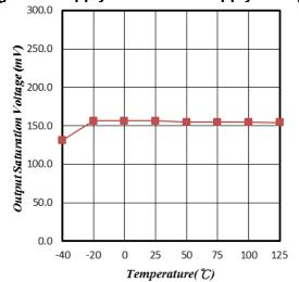
Figure 6. Output Saturation Voltage vs. Temperature
