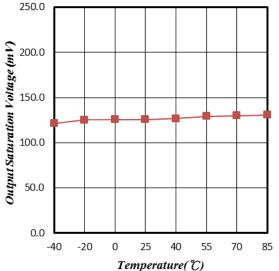
Figure 6. Output Saturation Voltage vs. Temperature
