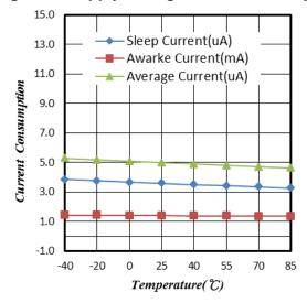
Figure 3. Supply Current vs. Temperature
