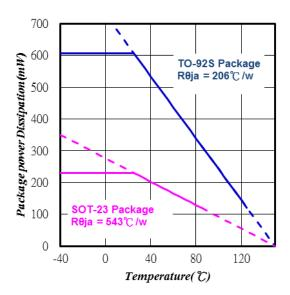
Figure 8. Power Dissipation vs. Temperature
