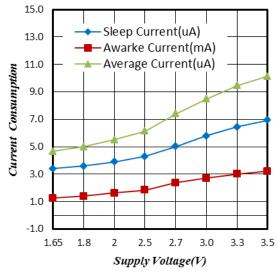
Figure 4. Supply Current vs. Supply Voltage
