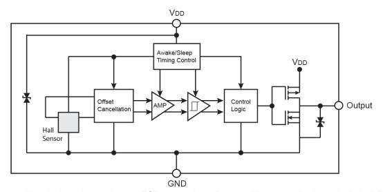
**Note:** Static sensitive device; please observe ESD precautions. Reverse  $V_{DD}$  protection is not included. For reverse voltage protection, a  $100\Omega$  resistor in series with  $V_{DD}$  is recommended.
