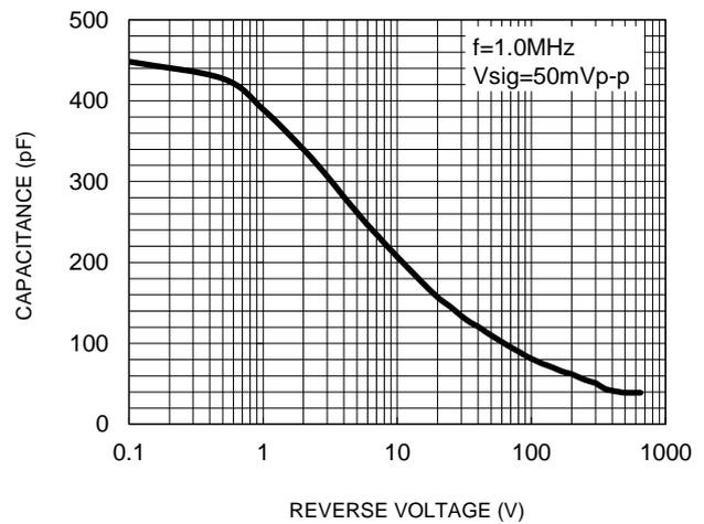
**Fig.5 Typical Capacitive Charge**
