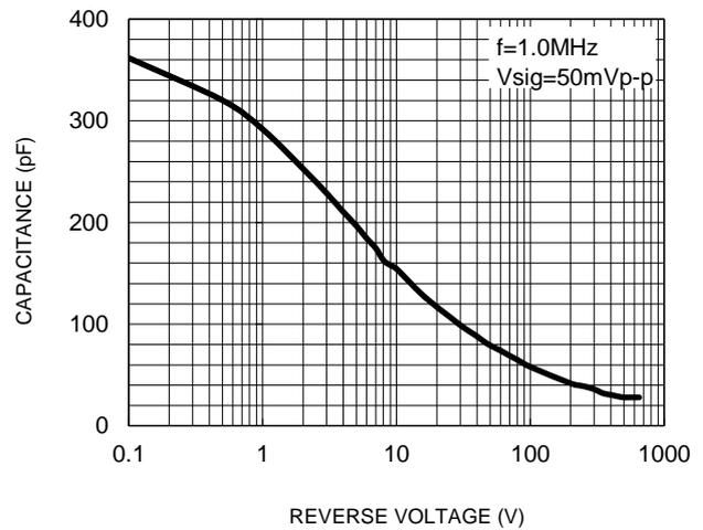
**Fig.5 Typical Capacitive Charge**
