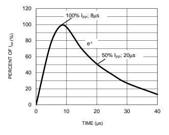
Fig.7 ESD pulse waveform per IEC61000-4-2
