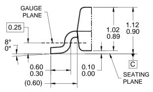
DETAIL A, ROTATED -90° (SCALE 2:1)
