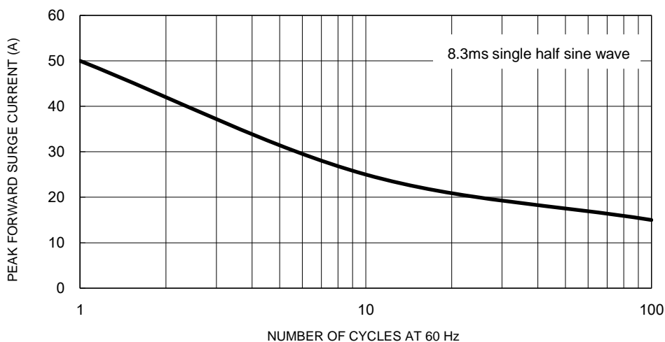
Fig.5 Maximum Non-Repetitive Forward Surge Current
