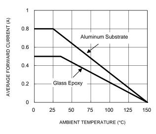
Fig.1 Forward Current Derating Curve
